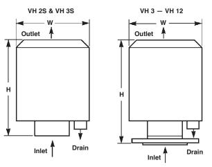
Inlet Connections: VH 2S is screwed 2" NPT; VH3S is screwed 3" NPT VH 3 — VH 12 flanged to suit ANSI 150 Flanges are the lap joint type.
