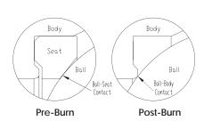
FIRE SAFE, Flo-Tite's Model T12 valves are supplied as standard with graphite stem packing and body seal. Valves are certified fire safe. In the event of a fire, after heat destroys the primary resilent seat, the ball makes contact with the secondary metal seat, forming a secure seal. The graphite body seal prevents external leakage. The graphite live-loaded stem packing prevents stem leakage. All valves have anti-static devices, grounding ball and stem to the body as standard.
