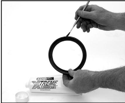
**1 CHECK & LUBRICATE GASKET—** Check gasket to be sure it is compatible for the intended service. Apply a thin coating of Guvlok lubricant to the exterior surface and sealing lips of the gasket. Be careful that foreign particles do not adhere to lubricated surfaces.
