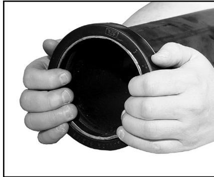
**2 GASKET INSTALLATION—** Slip the gasket over the pipe end making sure the gasket lip does not overhang the pipe end. On couplings 10" and larger it may be easier to turn the gasket inside out then lubricate and slide the gasket over the pipe end as shown.
