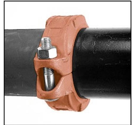
**6 ASSEMBLY IS COMPLETE—** Visually inspect the pipe joint to assure the coupling keys are fully engaged in the pipe grooves and the bolt pads are in firm even metal-to-metal contact on both sides of the coupling.
