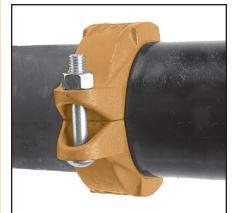
**6**Visually inspect the pipe joint to assure the coupling keys are fully engaged in the pipe grooves and the bolt pads are in firm even metal-to-metal contact on both sides of the coupling.
