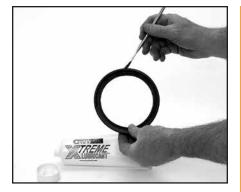
**CHECK & LUBRICATE GASKET**— Check gasket to be sure it is compatible for the intended service. Apply a thin coating of Gruvlok lubricant to the exterior surface and sealing lips of the gasket. Be careful that foreign particles do not adhere to lubricated surfaces.
